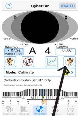
8. During the rest of this procedure, gently press the iOS device and CyberFork towards each other and against the padded surface, keeping them as still as possible. This minimizes the effects of air distortion, enabling the iOS device to “hear” the CyberFork’s pitch with virtually the same accuracy as a direct-line input. Accurate calibration is possible only in a noise-free environment, so find a peaceful quiet moment for calibrating.
